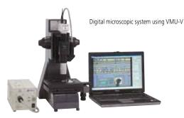
By installing a digital camera on a microscope the VMU provides a simple and compact system which allows microphotography and simultaneous external monitor observations. The VMU can be used in vertical and inverted positions according to your application requirements.
