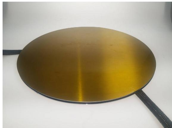
Figure 1. 300 mm Temperature Calibration Wafer
