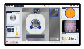
By implementing intuitive multi-touch operation, QAlibria® provides crisp and clear guidance to the RF calibration process, minimizes configuration mistakes and helps to reach accurate calibration results in fastest time. QAlibria® offers industry standard and advanced calibration methods.
