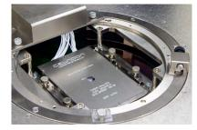
Celadon, high-performance, low-leakage probe cards
