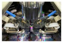
RF LTM probe arms, equipped with SmartCarrier™
