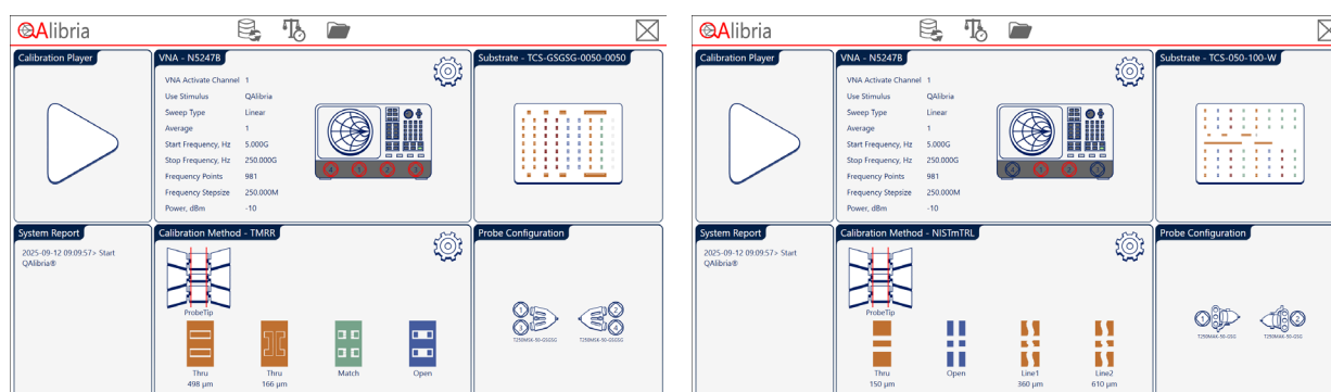
Example of QAlibria® user interface for calibrating the system with a TITAN™ Probe T250MSK-GSGSG0050 and T250MAK-GSG0050.
