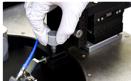
Figure 4. Planarization of TITAN™ Probes.
