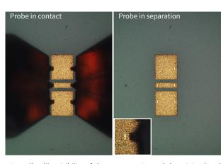
DC-needle-alike visibility of the contact point and the minimal pad damage due to the unique design of the tip
