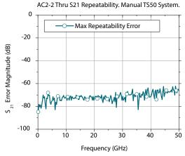
The maximal probe contact repeatability error of the calibrate S21-parameter of the AC2-2 thru standard by T50 probes. Manual probe system TS50.
