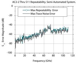
The maximal probe contact repeatability error of the calibrate S11-parameter of the AC2-2 thru standard by T110 probes. Semi-automated system. Ten contact circles.
