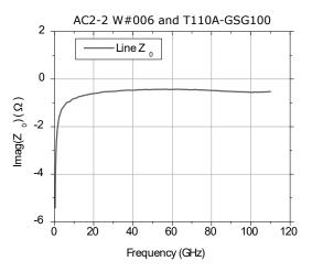
Typical characteristics of the coplanar line standard of AC2-2 calibration substrate measured using T110-GSG100 probes, and methods recommended by the National Institute of Standard and Technologies  $^{[2,\,3]}$ .
