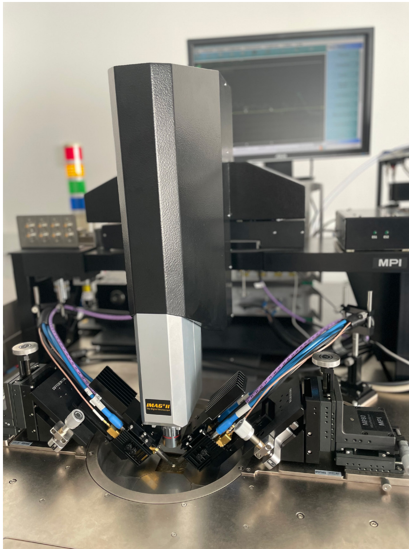
Fig. 1: Anritsu VectorStar ME7838G 70 kHz–220 GHz broadband VNA integrated with the MPA TS3500-SE system.
